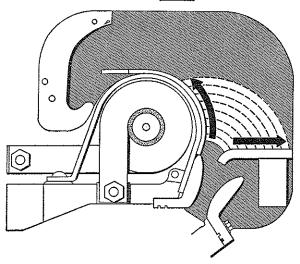
CAUTION—Before operating the contactor under load, be sure that the arc shield is lowered in its proper position.
