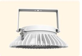
The HBLC Crane light is a specially designed light fixture for use on heavy industrial bridge cranes. It is typically mounted on the bottom of the bridge crane to light the area shadowed by the bridge crane body. The fixture can accept either 120v - 277v AC or 170v - 390v DC. A yoke mount is used for strength and mounting flexibility.
