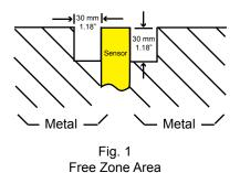
Select a mounting area, keeping the Free Zone requirements (Fig. 1) in mind. The target must move laterally across the face of the speed switch. Actuating distance from the target to speed switch face is shown in Fig. 4 and Table 5 (Page 3). The information provides an estimated setup distance prior to actual starting.
