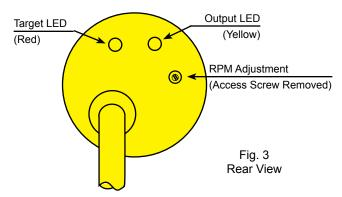
The Yellow output LED, Fig. 3, will light when the sensed speed is above the speed setting. The Yellow output light also signals that the output triac is on and shows that the series-connected load is actuated.
