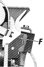
steel washer) is next to the coil. (Note that the coil spring washer (37) is positioned concave side towards the coil.)
