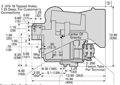
4-.250 Faston Tabs For Customer's 2-.375 -16 Tapped Holes, Terminals C-D & G-H Connections T0 Magnet Coil 1.0 (25.4) Deep, For Customer's Connection On Reverse Side
