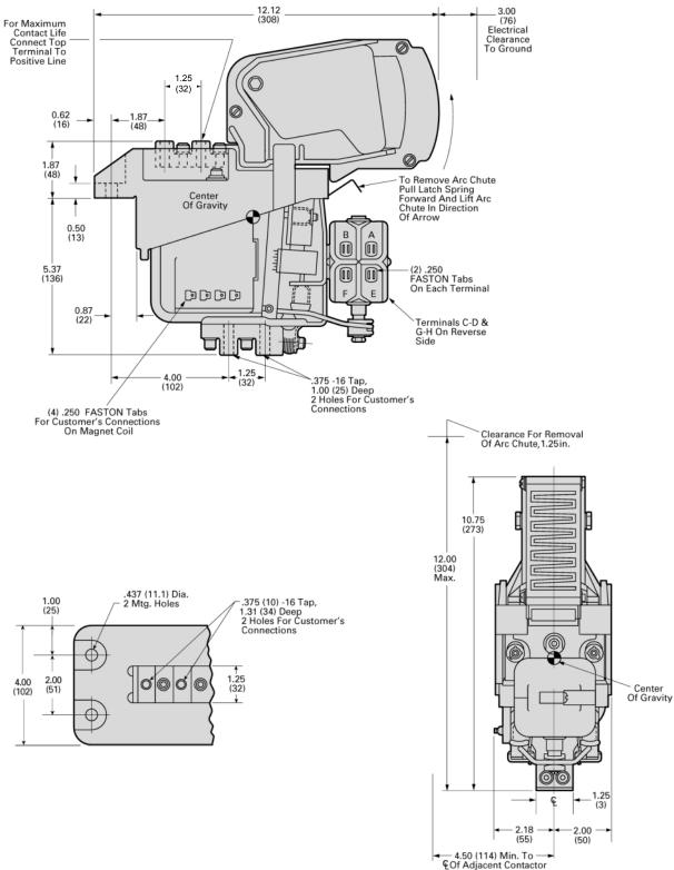
All dimensions shown in inches and (millimeters). For reference purposes only. Not to be used for design or construction purposes.
