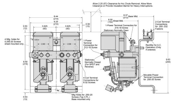
All dimensions shown in inches and (millimeters). For reference purposes only. Not to be used for design or construction purposes.
