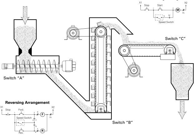
Illustration of Mechanical and Electrical Interlock uses of Speed Switches
