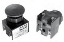
Hubbell's maintained pushbuttons are available in two variations. Single button mushroom head "push/pull" units are stand alone buttons that are commonly used for a maintained "emergency stop" function which has "push-to-stop/pull-to-start" operation. Single maintained buttons are used with another operator and an MRI "maintained reset interlock" to provide two button operation for either "maintained/maintained" or "maintained/momentary" action.
