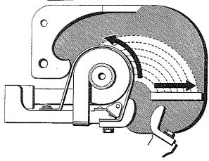
CAUTION - Before operating the contactor under load, be sure that the arc shield is lowered in its proper position.
