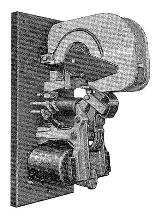
OPERATING COILS: These contactors will operate satisfactorily on 80% of normal control voltage when the coils are hot and will hold in on 20% of normal voltage. The coils will stand 110% of normal voltage continuously.
