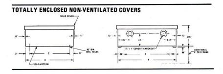
DC LIMIT SWITCH RESISTORS 230/250 VDC, ENCLOSED FOR USE WITH DYNAMIC LOWERING HOISTS
